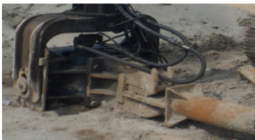
图3 桩顶金属套帽
