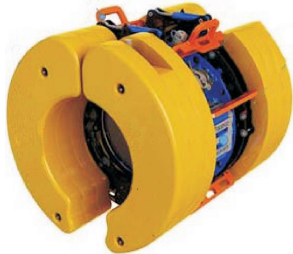
Figure 4. CT Scanner for Submarine Pipeline
