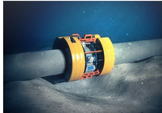
Figure 11. Working State of Pipeline CT Scanning
