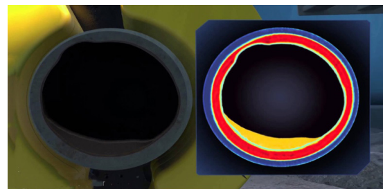
Figure 14. Hydrate Detection in Coated Pipes
