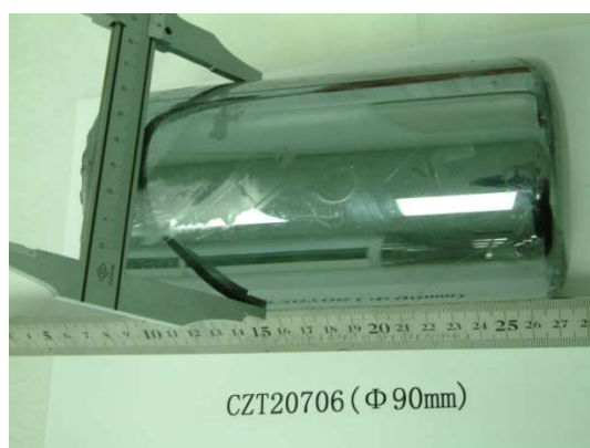
Figure 3. Growing \Phi 90mm CD1 xznxte crystal
